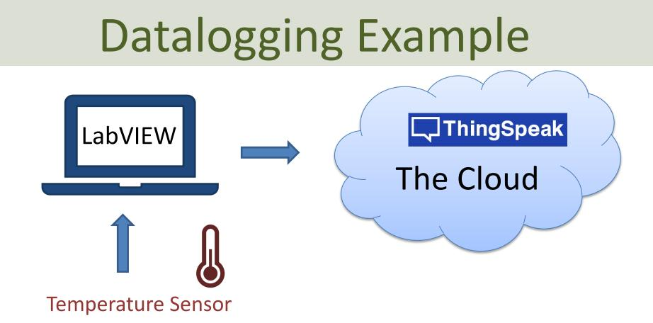
(In this Tutorial a TC-01 Thermocouple Temperature Sensor from National Instruments will be used, but any kind of sensor can be used)
